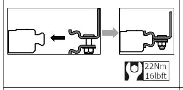
4. Fit the mounting brackets over the dovetail. Tighten to specified torque
